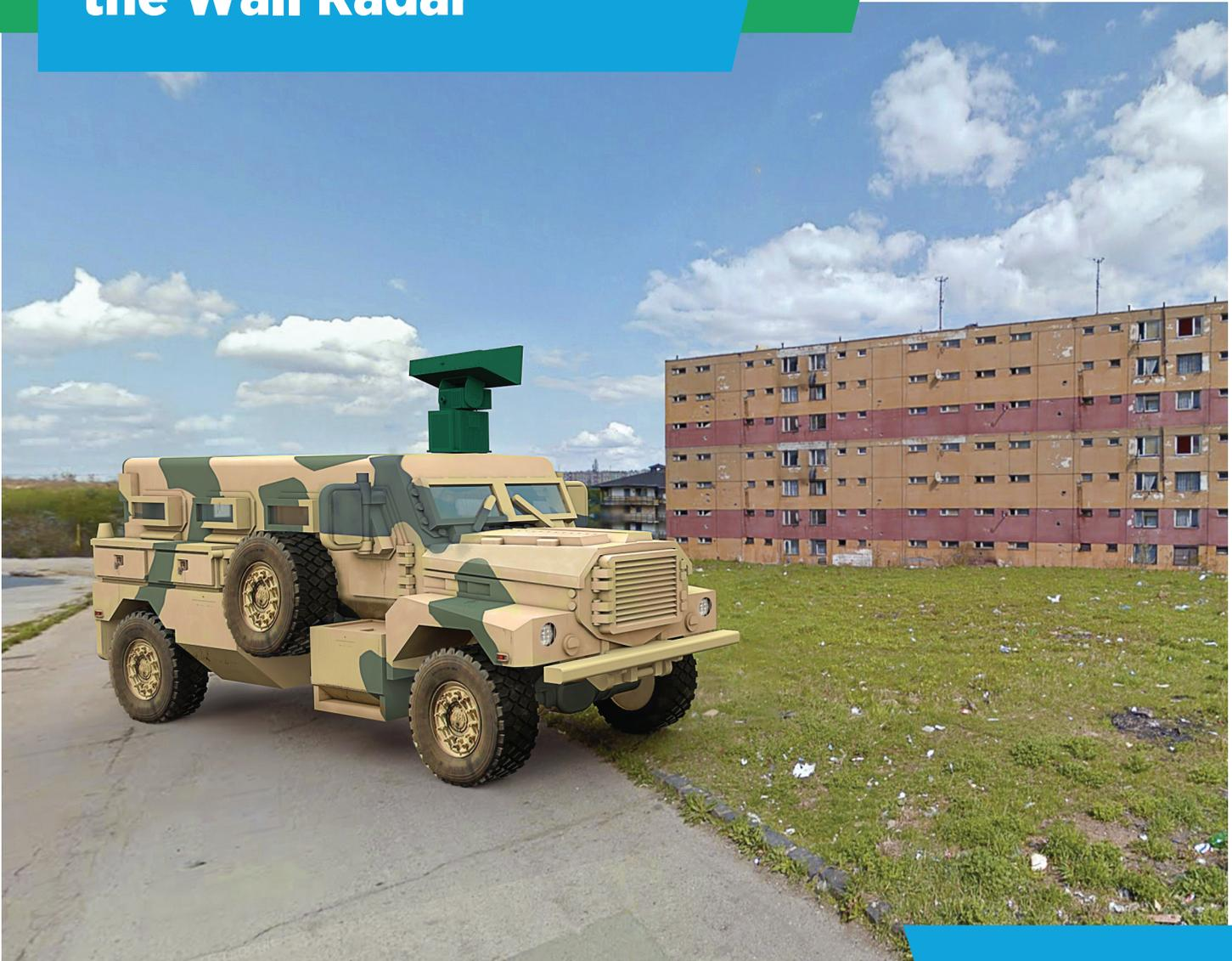
Standoff Through the Wall Radar (**UHTES**) is a through the wall imaging system that utilizes Ultra Wide Band (UWB) radio frequency signals to detect living beings beyond walls, obstacles and etc. from safer distances.
