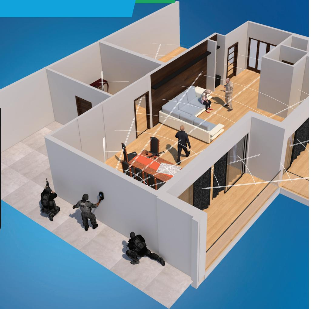
**m-DAR** (mini Through-the-Wall Radar) is a highly compact through-the-wall radar system which utilizes Ultra Wide Band (UWB) radio frequency signals to determine the distance of static and moving targets behind obstacles.
