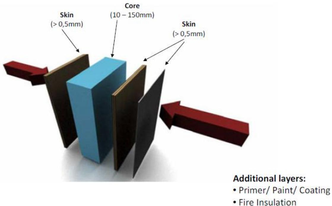
Figure 2.5. Composite layers (Wenstrom 2008)
