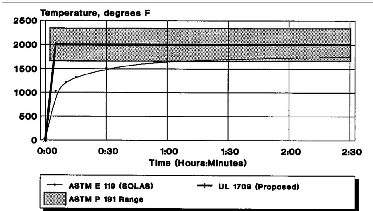
Figure 3.1. Comparisons of Three Fire Tests (Ship Structure Committee 1990)
