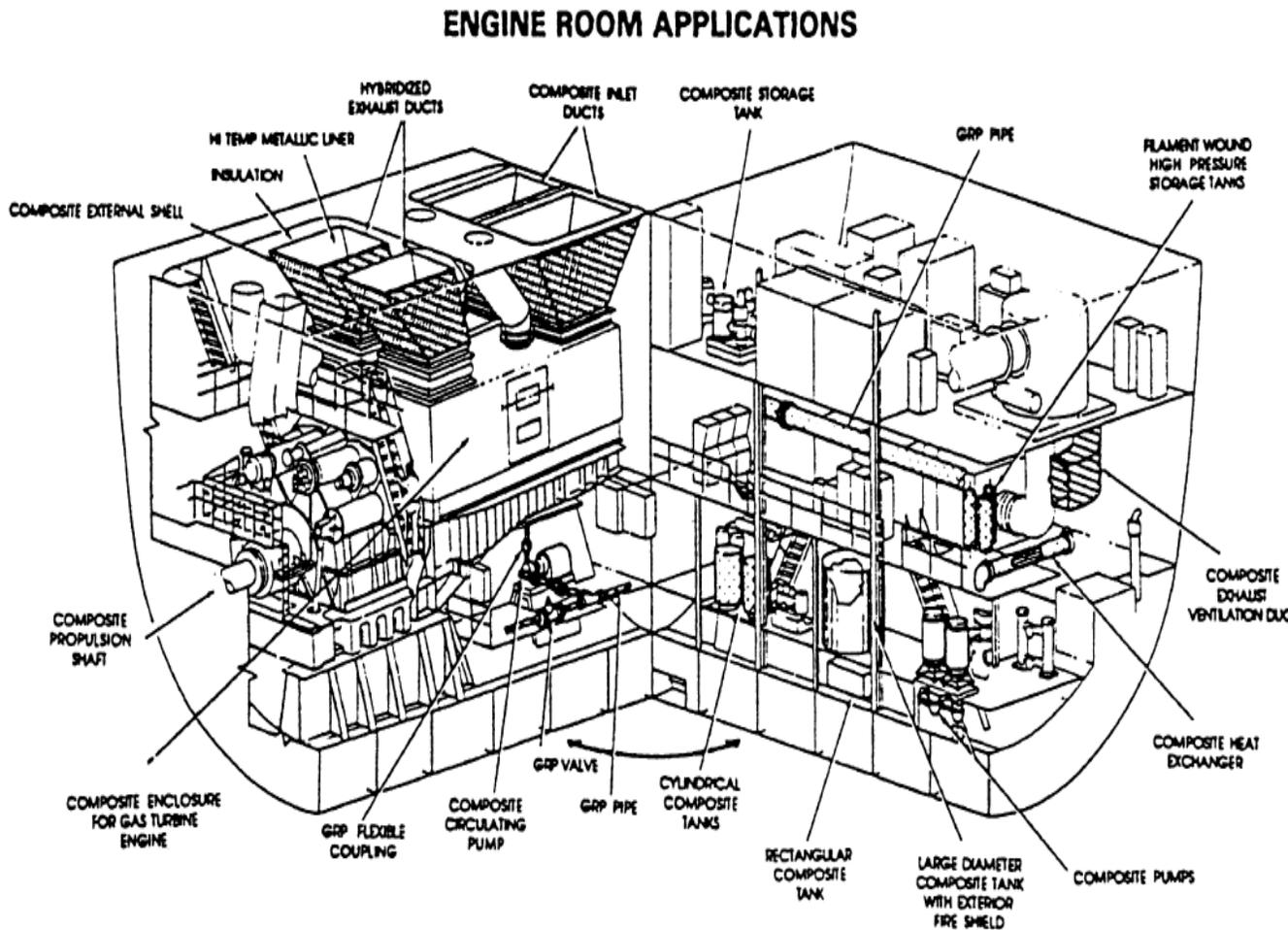
Figure 2.1. Applications for composites in ship machinery compartments (Mouritz 2001)
