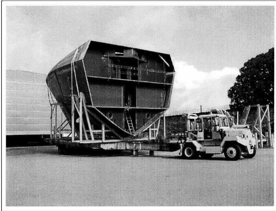
Figure 3.18. Bow section of the Visby-class corvette under transportation to the outfitting workshop ([www.canit.se](http://www.canit.se))
