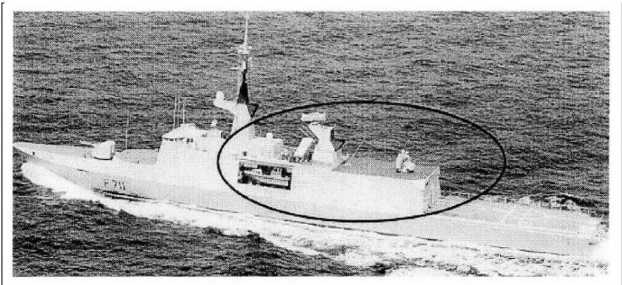
Figure 2.2. La Fayette frigates with the composite superstructure section. (Mouritz 2001)
