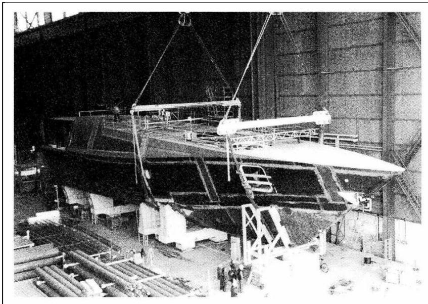
Figure 3.15. Sweden's YS2000 class corvette, the first known production naval at Kockums' shipyard on Karlskrona Island (Valenti 2001).
