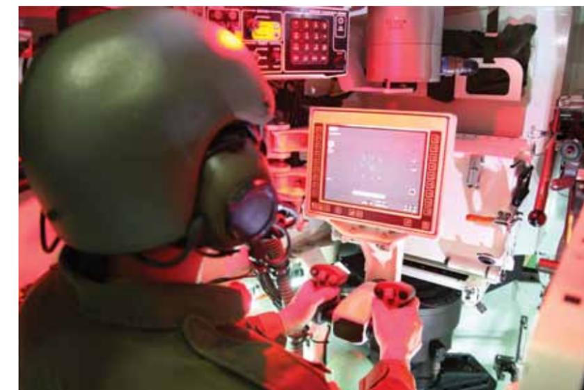
The MBT has many hardware and software configuration items each of which has their own distributed software architecture and the Vehicle Control System is the main gateway used to connect the systems to each other by means of Otokar's specially designed data interchange protocol.
