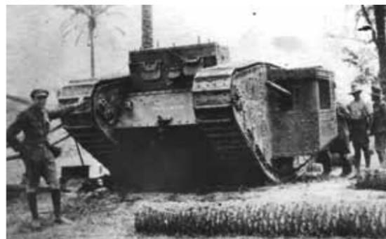
The idea was that if grenades were thrown onto the tank they would roll off again before they exploded, rather similar to the net and slat armour solutions integrated on board Mine Resistant Ambush Protected (MRAP) vehicles during the recent Iraq and Afghanistan campaigns, designed to stop rocket-propelled grenades.
