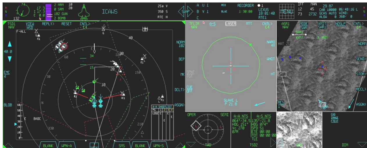
Fig. 1 Information fusion is a set of algorithms that combines data from all sources to create an integrated view of the environment.
