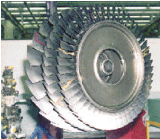
Figure 7: F110-GE-129 EFE assembled blisk fan rotor. The blisk fan produces reliability improvements over the current system by eliminating potential sources of high stress regions such as blade dovetails and mid span shrouds.
